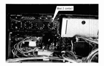
fig 2. Contact for mod 2 is at 12 o'clock position.
